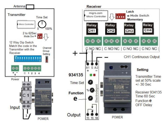
NOTE: Transmitter and Receiver antennas shall be mounted facing the same vertical position, (same polarity pattern) even when there is no line of sight.
